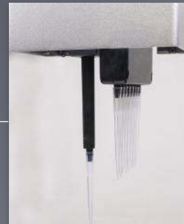
Flexibility with two parallel pipette mounts (any combination of single- and 8-channel)
