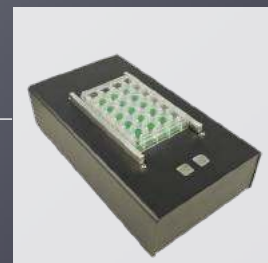
Integrated MEA amplifier in pipettor's baseplate
